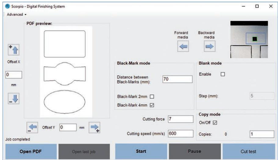
The Scorpio is equipped with a camera used to detect the black-mark printed on the media. This camera assist the software in detecting the black-mark created inside the cutting file.
